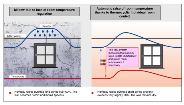
The THZ individual room control regulates room temperatures depending on humidity to avoid mildew.
